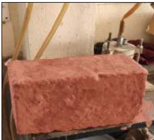
Figure 3: Brick's filled with mixture of Nano Silica and Bio mineral
