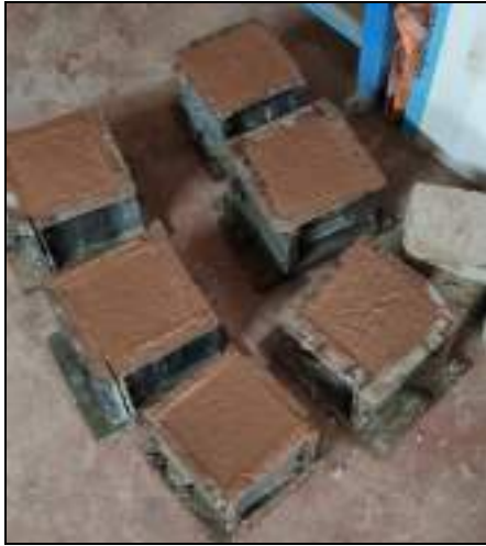
Figure 5: Laterite blocks kept in mould
