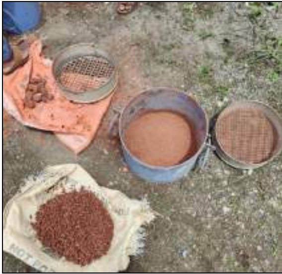
Figure 5:Crushing of laterite brick, Fine aggregates <4.75mmCoarse aggregates >4.75mm
